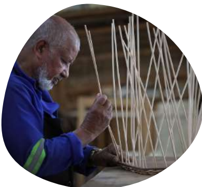
An SBU fitting the stakes to start weaving
